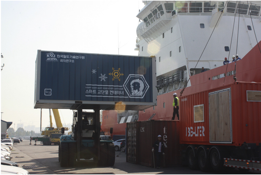
Figure 7.1 The high-insulated container developed by KRRI. KRRI, Korea Railroad Research Institute.
