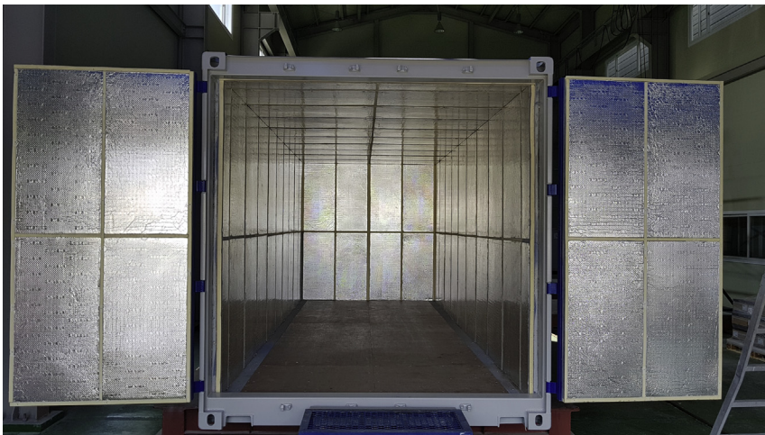
Figure 7.2 Inside of the high-insulated container.
